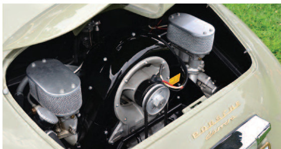
>>> Ben and Rob Edwards' four-cam power plant. One of three four-cam cars at the show.
