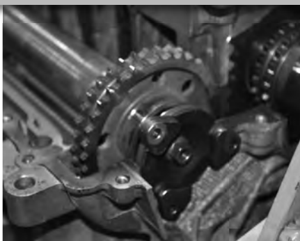
>>> Force is applied to the tool to extract the bearing
