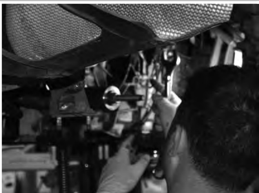
>>> Force is applied to the tool to extract the bearing
