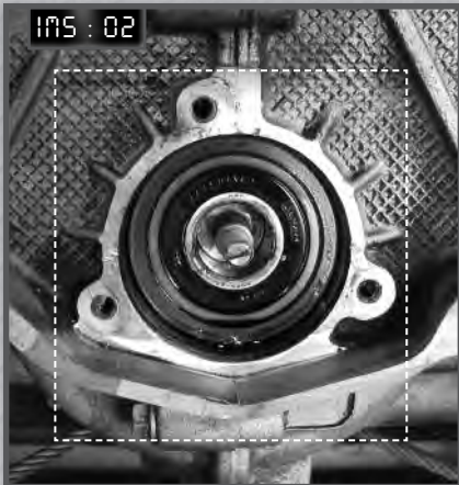
This particular motor is an early version and utilizes a double row version of the bearing. Special tools are required to extract the inner bearing and remove the inner bearing race retainer, actually destroying the retainer in the process.
